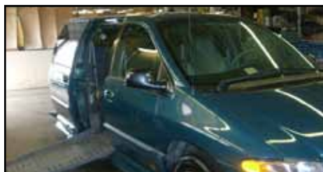
2000 Dodge Grand Caravan SE. Braun Entervan Conversion with a 10" lowered floor. Automatic side entry with power kneel, door, and ramp. 6 way drivers side transfer seat, removable front passenger seat. 4 way tie downs and lap belts. 800-420-6470 OCT V18
