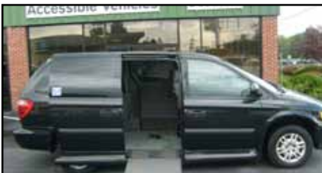
2005 Dodge Grand Caravan SXT/VMI Northstar Conversion. 10" lowered floor. Auto. kneel system, door, and ramp. Removable front passenger seat. 4 pt. tie downs w/ lap belts. 6 way driver transfer seat, with MPD Handcontrols. EZ Lock mid ship section. 800-420-6470 OCT V19
