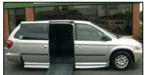
2002 Dodge Grand Caravan Sport. With Braun Entervan II Conversion, 8" lowered floor, Power kneel system, door, and ramp with hand held remote operation. Removable driver and front passenger seats. Multiple mounting strips, tie downs, and lap belts. 800-420-6470 OCT V20
