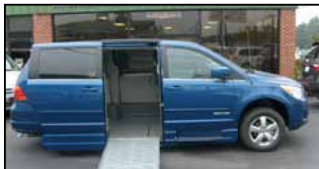
2011 Volkswagen Routan SE. W/ an American Wheelchair Conversion, 14" lowered floor. Power kneel, door, side entry ramp. Removable front driver/passenger seats. Multiple interior switches.. Fold/flip foot rest. 56" door height. 57 1/2" Inside height. Multi-trac tie down attachments, tie downs, and lap belts. 800-420-6470 OCT V27
