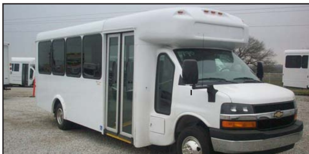
2011 Arboc Spirit of Freedom. Low Floor unit with WC ramp. Driver plus 23 passengers or 17 passengers and 2 WC positions. Priced below cost to move out of inventory. Call Andrew Clawson (540)256-3246 for pricing. OCT V31
