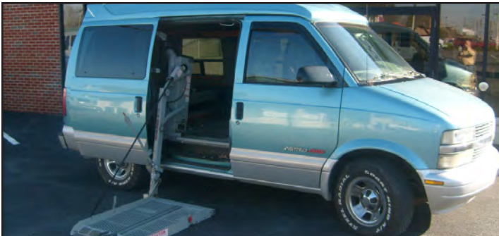
1995 Chevrolet Astro AWD. Mid size van with raised roof, power lift, door, and transfer seat. Outside door toggle switch. Door entrance 44.5" and Midship height 55.5". Tilt steering and cruise. Dark tinted glass. Call for a demo and pricing. 1-800-420-6470 JAN V30
