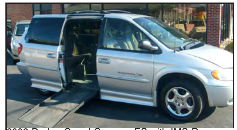
2002 Dodge Grand Caravan ES with IMS Rampvan side entry conversion. 10" lowered floor, Power kneel, door, and ramp. Hand held key fob. Driver's 4 way transfer seat. Removable front passenger seat. $9,500. Call 800-420-6470 JAN V12
