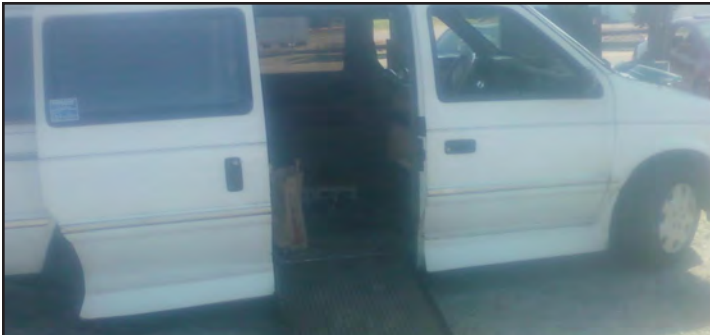
1993 Dodge Grand Caravan with Rollx Manual Conversion. Includes four point tie downs, 10 inch lowered floor, manual passenger side door, manual ramp. Removable front passenger and driver's seat. Call 1-800-420-6470 JAN V9
