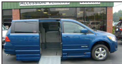
2011 Volkswagen Routan SE. W/ an American Wheelchair Conversion, 14in lowered floor. Power kneel, door, side entry ramp. Removable front driver/passenger seats. Multiple interior switches. Fold/flip foot rest. 56in door height. 57 1/2in inside height. 800-420-6470 JAN V25
