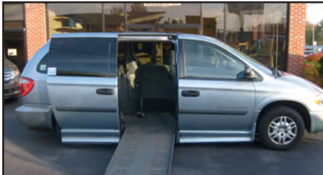
2005 Dodge Grand Caravan with Braun Rampvan Conversion, 10in lowered floor, power kneel, ramp, and door. Removable driver & front passenger seats. Multiple mounting plates and retractable tie downs. Fully automatic chassis. 540-932-7300 DEC V24
