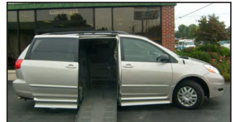
2009 Toyota Sienna LE. Braun Entervan side entry ramp, 10 in. lowered floor. Power kneel, door, and ramp. Multi-trac tie down attachment straps and lap belts. 800-420-6470. DEC V27
