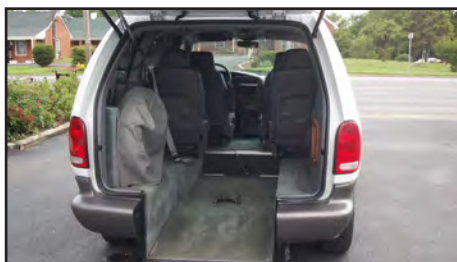
1997 Plymouth Grand Voyager Se/Viewpoint rear entry conversion. 8" drop floor, remounted mid-ship seats. Power rear hatch and ramp. EZ Lock and 4pt tie downs with lap belts. 68K Mi. 800-420-6470 JUNE V10
