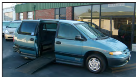
1996 Dodge Grand Caravan IMS Handicap Accessible Van Conversion. 8 in. lowered floor, 4 pt tie downs. Power door/ramp/kneel system. Removable passenger seat. Driver 6 way transfer seat. MPD handcontrols. On board trickle battery charger. 800-420-6470 JUNE V12
