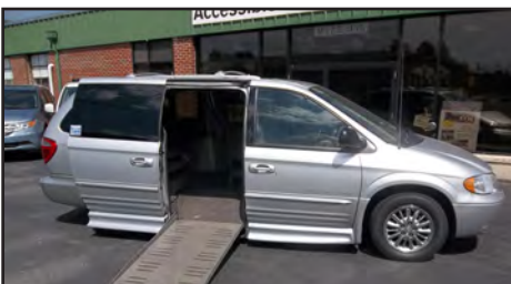
2003 Chrysler Town & Country Limited Braun Entervan II Conversion, 10" Lowered floor, Power side entry ramp. Removable driver & passenger seat. 4 point tie downs, and lap belts. 800-420-6470 JUNE V16
