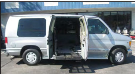
2001 Ford E 150 with a Braun Vangater II Lift. 6" lowered floor, Automatic doors with dash mounted, exterior magnetic, and hand held remote entry. 8 way driver transfer seat and EZ out passenger seat. 4 point tie downs and lap belts. Call 1-800-420-6470 for details. JUNE V4
