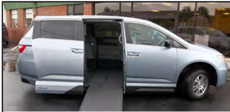
2011 Honda Odyssey EX L Res with VMI's Northstar Infloor Ramp Conversion: Full 10" lowered floor, Power kneel, door, and ramp. Multi-trac mounting plates, Q-strains, lap, and shoulder belts. EZ out driver and front passenger seats. VMI's Sure deploy back up system. Call for a demo today! 1-800-420-6470 JUNE V25
