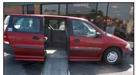
1999 Ford Windstar with an IMS side entry conversion. Lowered floor. Removable driver and front passenger seat. 4 point tie downs with lap belts. 800-420-6470 JUNE V11
