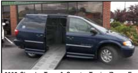
2005 Chrysler Town & Country Touring/Braun Entervan Conversion: 10" lowered floor, Power kneel system, door, and ramp. Removable driver/front passenger seat. Multi position tie down mounting plates. Dark tinted glass, DVD Entertainment package, Overhead console. 77K Mi. 800-420-6470 AUG V14
