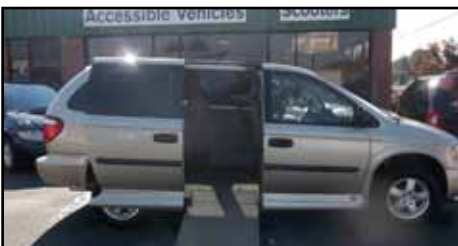
2005 Dodge Grand Caravan with VMI's Northstar Conversion. 10" Lowered Floor, Power Kneel Suspension, Side Sliding Door. Power In Floor Ramp. Removable Driver and Front Passenger Seats. 4 Point Tie Down Mounting Plates. Only 36K Miles. 800-420-6470. AUG V38
