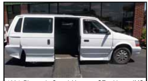
1994 Plymouth Grand Voyager SE with an IMS Rampvan conversion. 10" lowered floor, removable driver and front passenger seats. Automatic sliding door, kneel and ramp. External key switch entry. 4 pt. tie downs and lap belts. 540-932-7300 AUG V5
