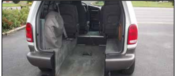
1997 Plymouth Grand Voyager Se/Viewpoint rear entry conversion. 8" drop floor, remounted mid-ship seats. Power rear hatch and ramp. EZ Lock and 4pt tie downs with lap belts. 68K Mi. 800-420-6470 AUG V8
