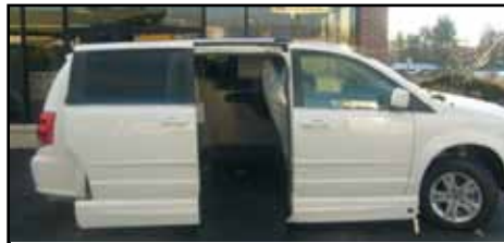
2011 Dodge Grand Caravan Crew featuring a VMI Northstar Conversion. 10 in. lowered floor, Auto. kneel, in-floor ramp, and side door. Removable driver and front passenger seats. 4 pt. tie downs and lap belts with multi mounting plates. 33 miles. Call for a demo today! 800-420-6470 AUG V17
