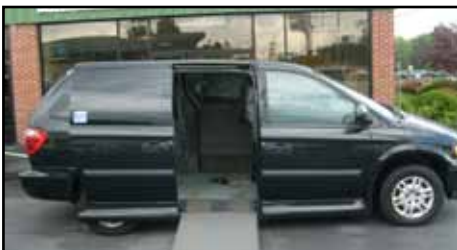
2005 Dodge Grand Caravan SXT/VMI Northstar Conversion. 10" lowered floor. Auto. kneel system, door, and ramp. Removable front passenger seat. 4 pt. tie downs w/ lap belts. 6 way driver transfer seat, with MPD Handcontrols. EZ Lock mid ship section. 800-420-6470 SEPT V16
