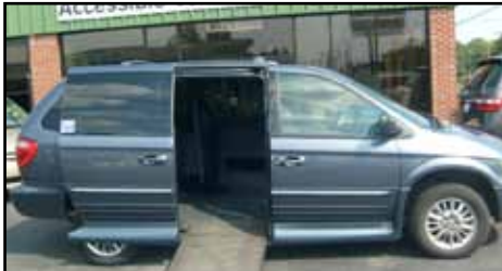
2002 Chrysler Town & Country Limited. VMI Northstar Conversion, with 10" lowered floor, power kneel, ramp, and door. Removable driver and front passenger seats. 4 way tie downs mounting plates. Electric park brake. 800-420-6470 SEPT V22
