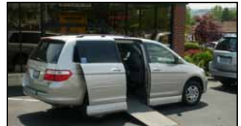
2007 Honda Odyssey EX/VMI Northstar Conversion. 10" lowered floor, kneel system, power door, and in floor ramp. Removable front seats. 4 pt. tie downs & multiple mounting plates. Magnetic and remote entry system. Multiple interior switches. 44K Mi. 800-420-6470 SEPT V25
