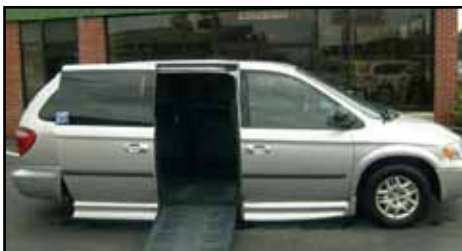
2002 Dodge Grand Caravan Sport. With Braun Entervan II Conversion, 8" lowered floor, Power kneel system, door, and ramp with hand held remote operation. Removable driver and front passenger seats. Multiple mounting strips, tie downs, and lap belts. 800-420-6470 SEPT V17
