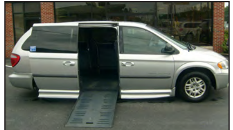
2002 Dodge Grand Caravan Sport. With Braun Entervan II Conversion, 8 in lowered floor, Power kneel/door/ramp with hand held remote operation. Removable driver and front passenger seats. Multiple mounting strips, tie downs, and lap belts. 800-420-6470 SEPT V14
