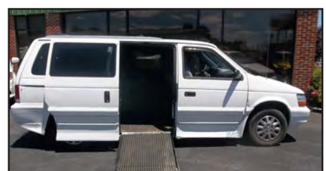
1994 Plymouth Grand Voyager SE with an IMS Rampvan conversion. 10" lowered floor, removable driver and front passenger seats. Automatic sliding door, kneel and ramp. External key switch entry. 4 pt. tie downs and lap belts. 540-932-7300 SEPT V8
