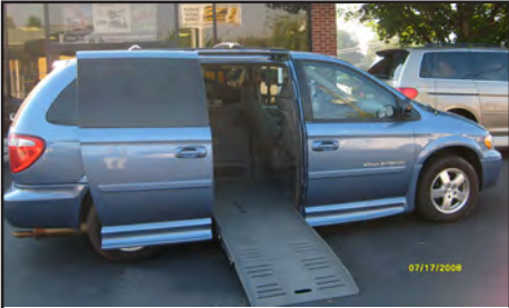
2007 Dodge Grand Caravan SXT. Braun Entervan conversion, remote entry, 10 in. lowered floor, power kneel, door, ramp. Removable driver and passenger seat. 4 way restraint system. 800-420-6470. SEPT V16
