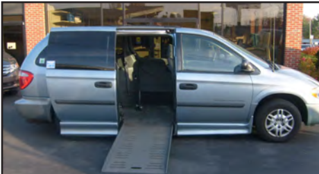
2005 Dodge Grand Caravan with Braun Rampvan Conversion, 10in lowered floor, power kneel, ramp, and door. Removable driver & front passenger seats. Multiple mounting plates and retractable tie downs. Fully automatic chassis. 540-932-7300 SEPT V15
