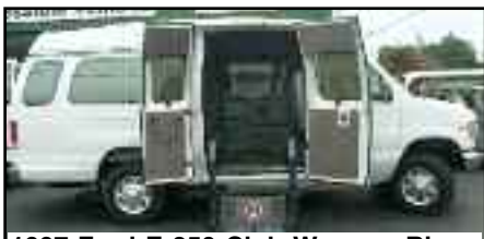
1997 Ford E 350 Club Wagon. Ricon S Series walk thru lift. 4 in. midship drop floor, removable front driver seat, tie down plates and retractable tie downs. Anti skid floor wheelchair area. 8 in. raised door panels, 63 in. entrance height. 12 in. raised roof and 68 in. head room height. 540-943-3430 DEC V29
